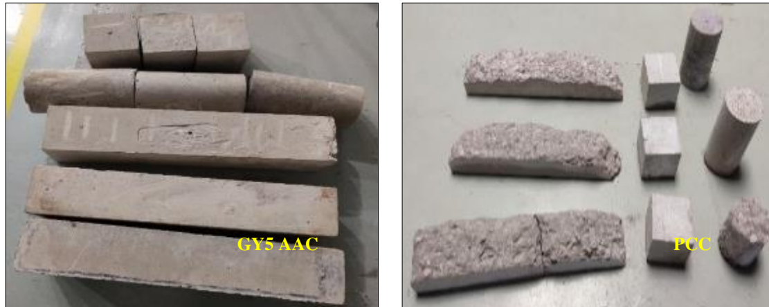
Figure 5. Concrete specimens after exposure to 800°C
