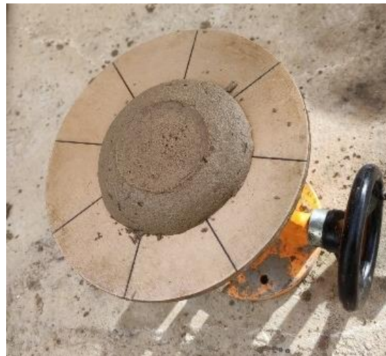
Figure 4. Execution of Flow Table Test
