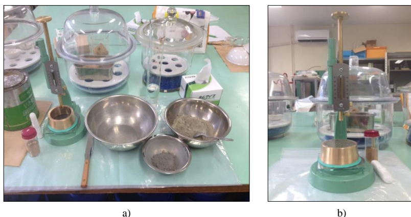
Figure 3. Examination of setting time of concrete: a) preparation of mass with standard consistency, b) examination with Vicat needle
