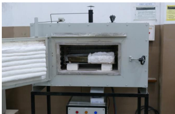
Figure 5. Electrical furnace for post-fire tests
