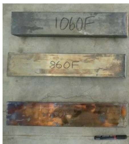
Figure 9. Post-fire test on RCFSSST columns
