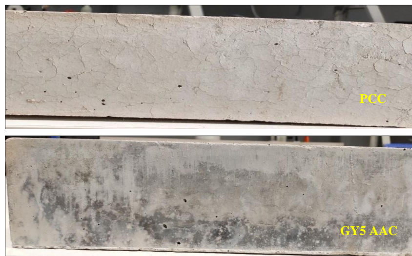
Figure 6. The visual appearance of G5 AAC and PCC beam specimens after exposure to 400°C
