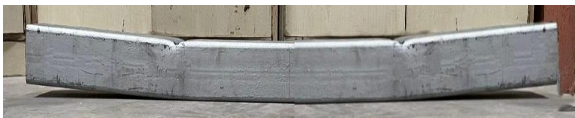
Figure 27. Failure pattern of beam in experimental study
