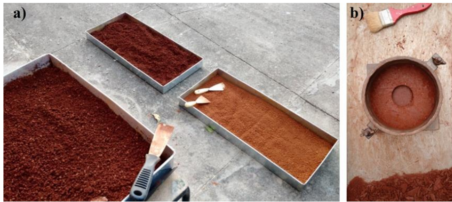
Figure 1. a) Samples with different water content. b) CBR specimen after performance of unsoaked CBR
