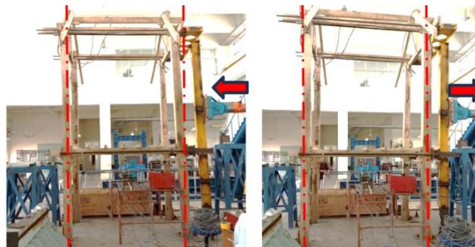
Figure 11. Deformation of the structure of wooden stilt houses
