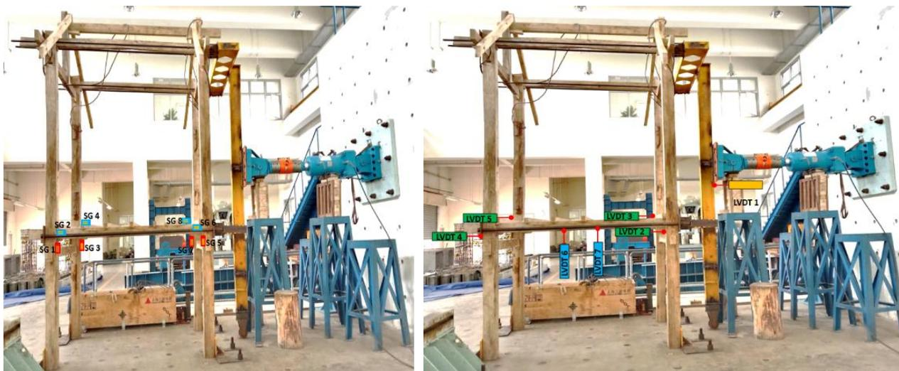
Figure 8. Placement of testing instruments (strain gauge) and LVDT
