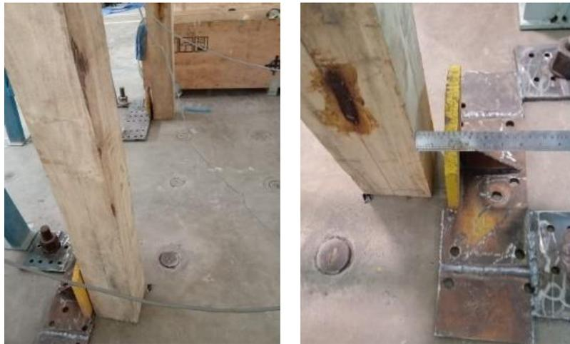
Figure 12. Translation of columns during testing, (a) before testing, (b) after testing
