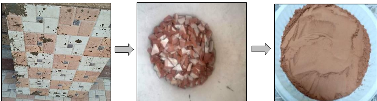
Figure 2. Transferring of Waste Ceramic Tiles (WCT) to Ceramic Powder (CP)
