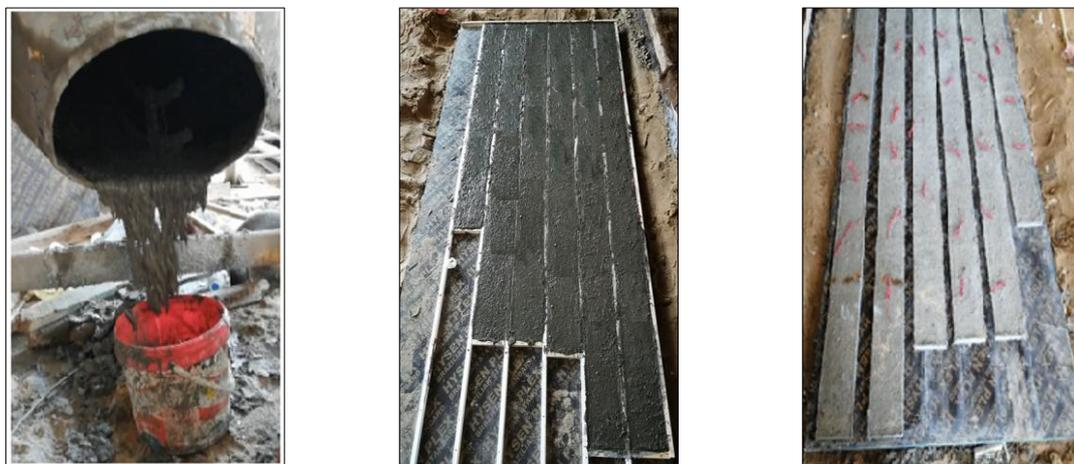
Casting the cementitious composite materials    Composite plate after hardening (Plain)    Composite plate after hardening (Strengthened)
