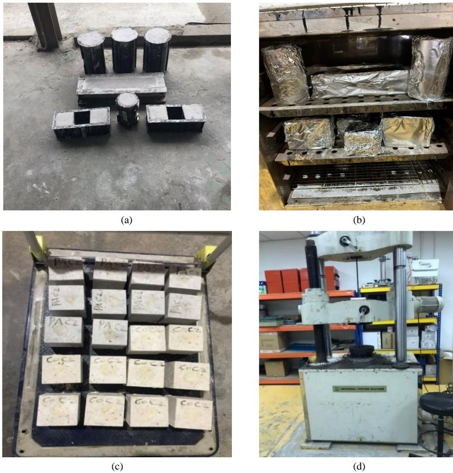
Figure 4. (a) the samples during casting, (b) the samples during steam oven curing, (c) the samples after casting, and (d) the Universal Testing Machine
