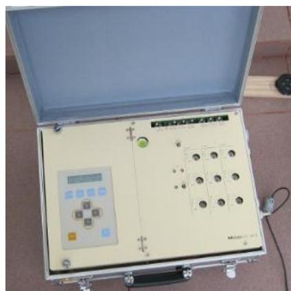
**Figure 4. The microtremor measuring instrument**
