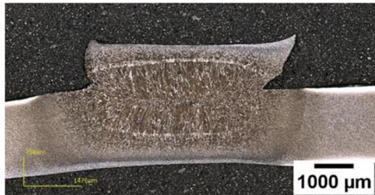
Figure 17. Representative button pull-out failure mode encountered after the tensile tests for all the samples
