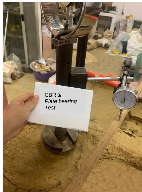
Figure 4. CBR and plate bearing test of the subgrade layer model in the laboratory
