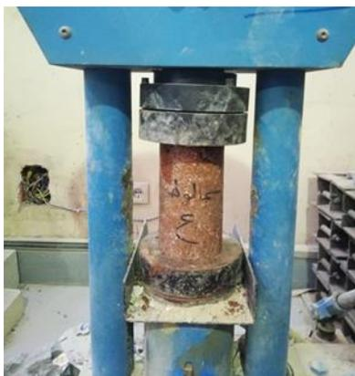
Figure 8. Compression test of core sample
