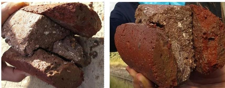
Figure 7. Complete separation observed between the mortar and bricks in
