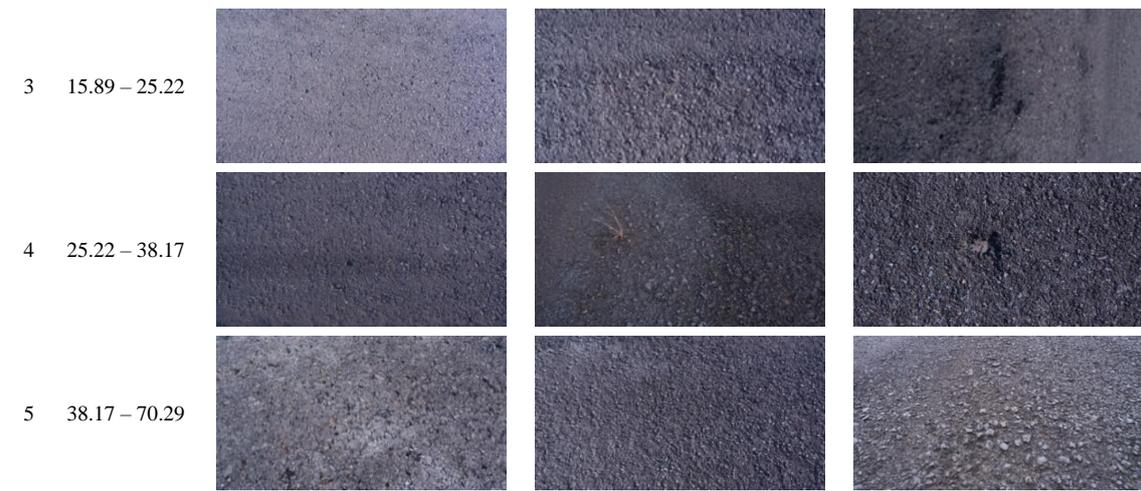
Another dominant type of damage was patching, a form of handling damage that occurred on airport pavements. Density classes could be grouped into five classes with a maximum damage density level reaching 13.96% of the sample unit area of 450 m<sup>2</sup>. Table 4 further showed examples of photo documentation of the damage divided according to density class and level of damage.
