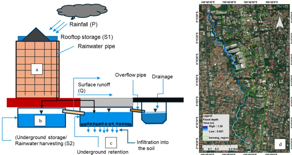
**Figure 14. Proposed NBS model for flood risk reduction; rooftop storage (a), underground storage (RWH) (b) and underground retention (c) in Kemang region and captured image after it applied in each sub basin in Kemang region (d)**
