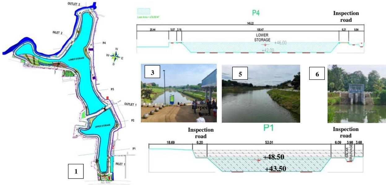
Figure 3. Layout of Brigif reservoir site (1), cross-section of Brigif upper storage (2), site view of Brigif upper storage (3) cross-section of Brigif lower storage (4) Site view of lower Brigif (5) and water gates of outlet Brigif reservoir (6)
