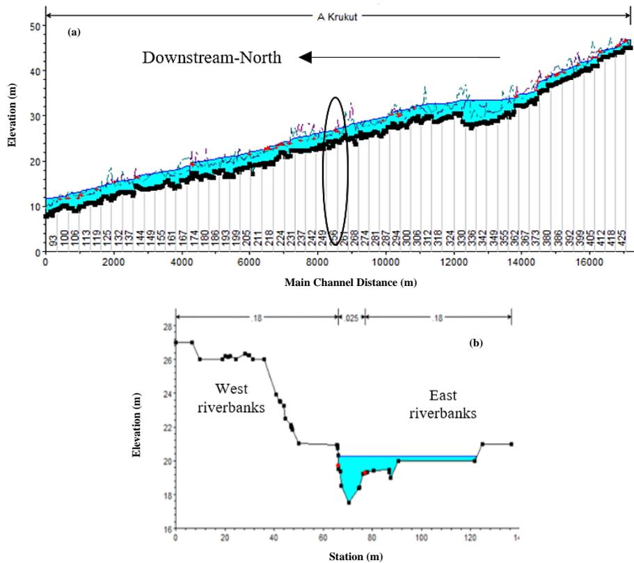
Figure 7. A long section profile of Krukut Watershed (a) and cross-section at Kemang region (b)
