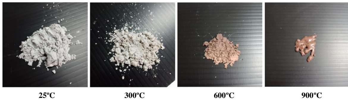
Figure 14. AGP after being exposed to 25°C, 300°C, 600°C, and 900°C
