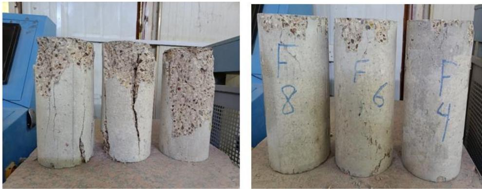
Figure 7. Compressive strength test (a) during test (b&c) after test (b) control mix (c) fiber mix
