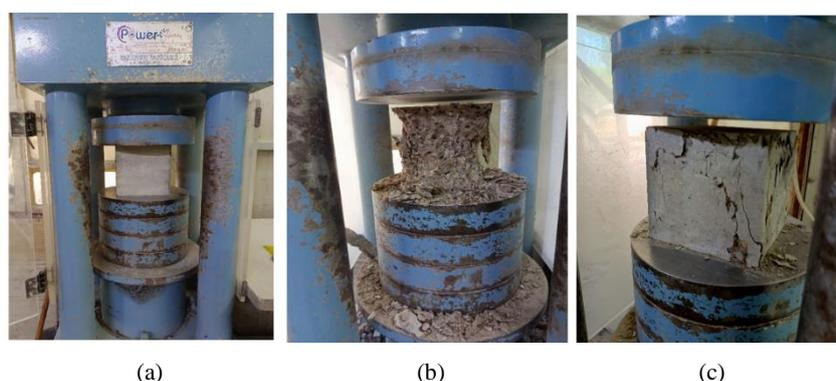
Figure 6. Cube compressive strength test (a) during test (b&c) after test (b) control mix (c) fiber mix
