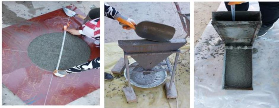
(a) slump flow and  $T_{50}$  test                      (b) the V-funnel test                      (c) L-Box test
