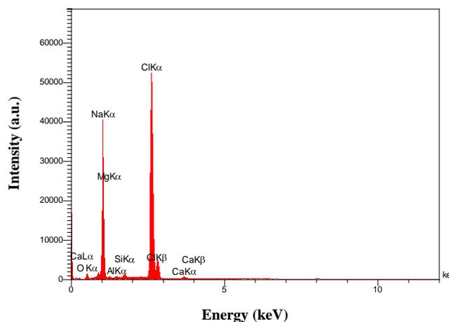
Figure 6. EDX-spectrum analysis for 7-days soaking period
