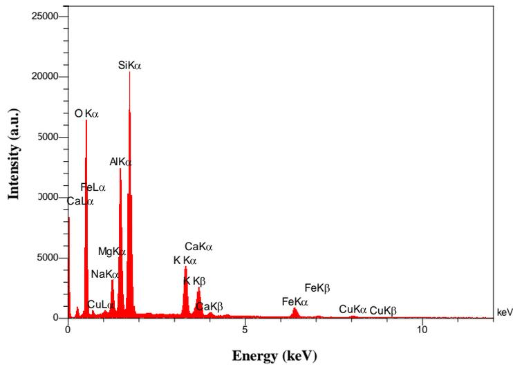
Figure 8. EDX-spectrum analysis for 30-days soaking period
