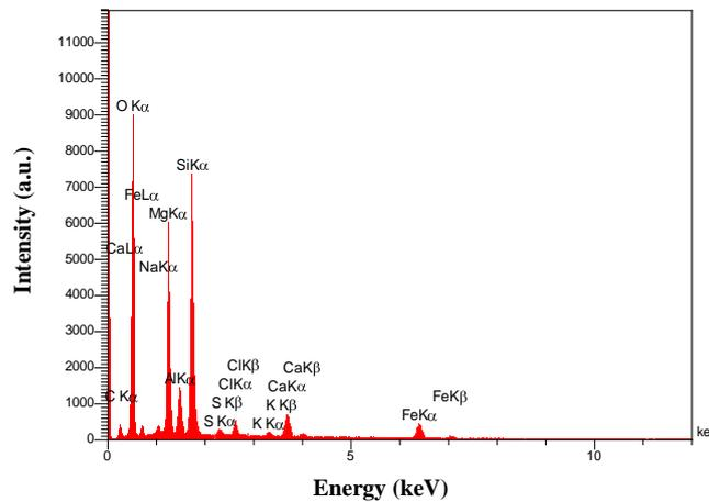
Figure 5. EDX-spectrum analysis for sample of dry soil
