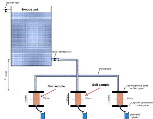
Figure 3. Device for the soil sample under soaking and seepage conditions
