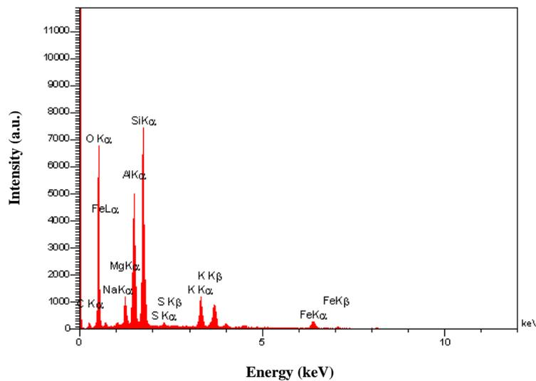
Figure 11. EDX-spectrum analysis for 30-days seepage period
