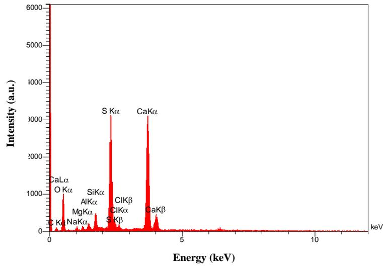
Figure 7. EDX-spectrum analysis for 15-days soaking period
