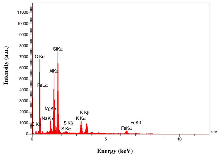
Figure 9. EDX-spectrum analysis for 7-days seepage period
