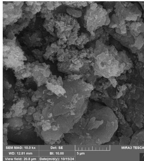
**Figure 14. SEM photo for dry soil sample**
