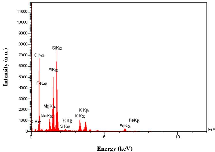
Figure 10. EDX-spectrum analysis for 15-days seepage period
