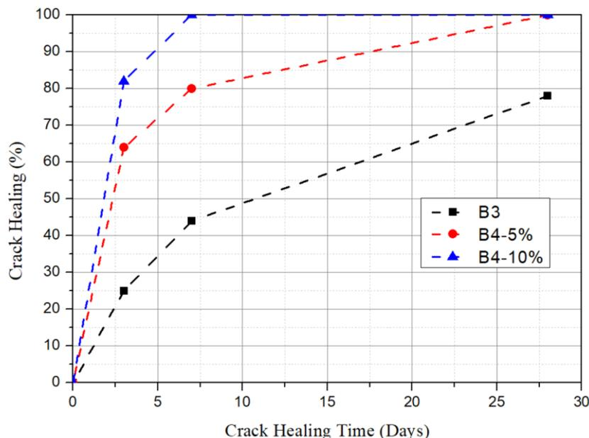
Figure 8. Percentage healing of cracks with respect to time
