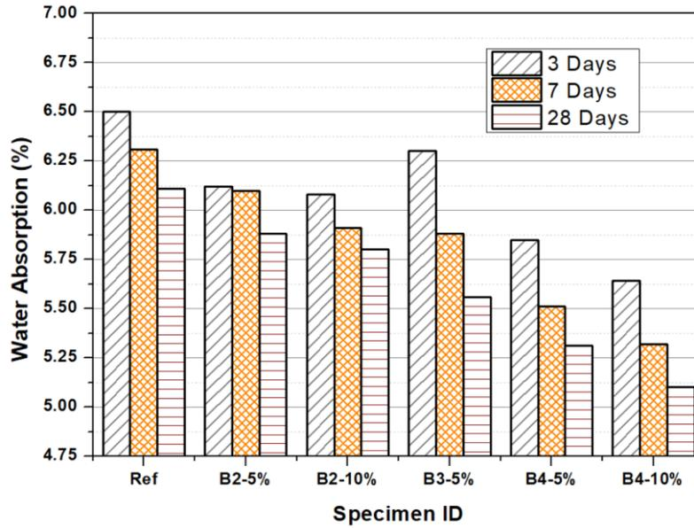
Figure 7. Percentage water absorption
