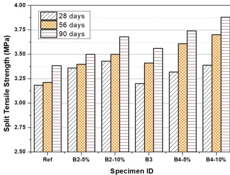
Figure 6. Split Tensile Strength
