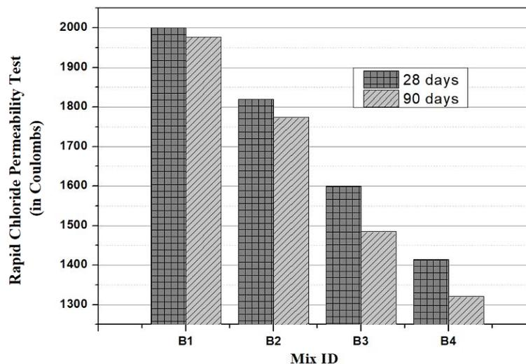
Figure 10. Rapid Chloride Permeability
