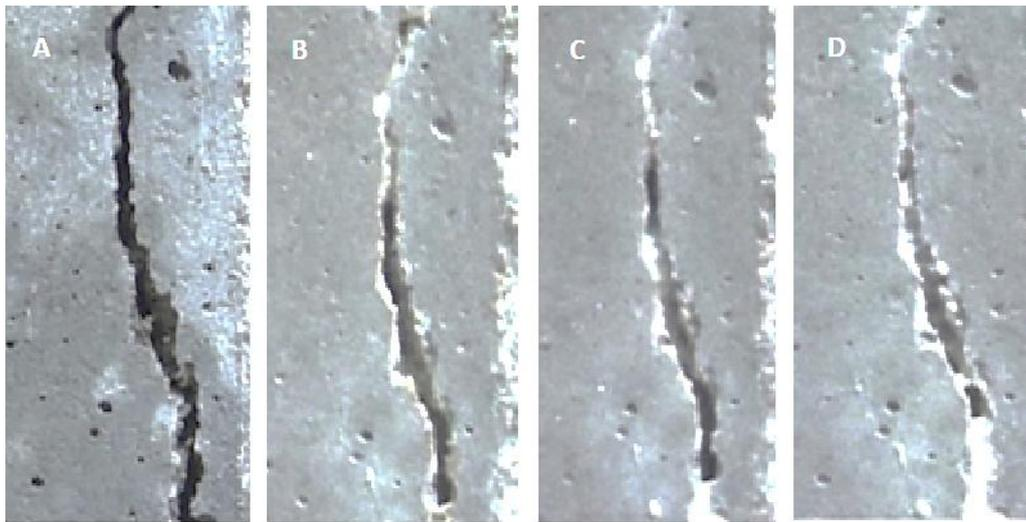
Figure 9. (a) 1<sup>st</sup> of crack, (b) 3<sup>rd</sup> day of crack healing, (c) 7<sup>th</sup> day of crack healing, (d) 28<sup>th</sup> day of crack healing for B3 mix
