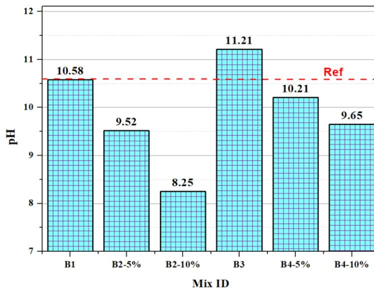
Figure 4. pH level of fresh concrete of different concrete mix
