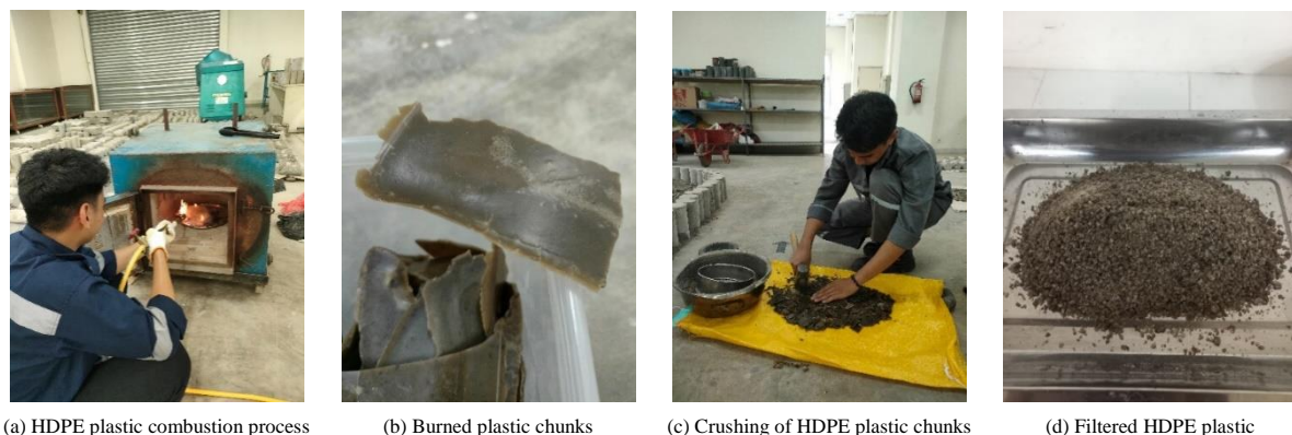
Figure 4. Process of converting HDPE plastic bag waste into a sand substitution material
