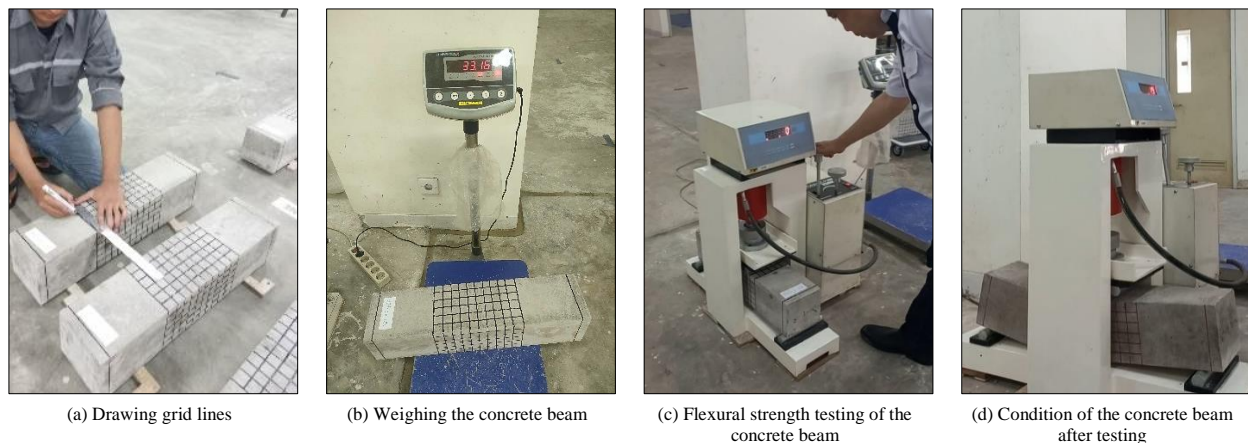
Figure 9. Stages of flexural strength testing process for concrete beams in the laboratory
