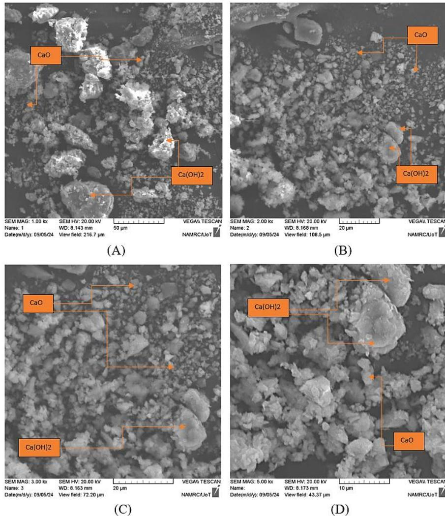
**Figure 14. SEM micrograph of soil with 5% quicklime. (A) Image captured at 1000x magnification. (B) Image captured at 2000x magnification. (C) Image captured at 3000x magnification. (D) Image captured at 5000x magnification**
