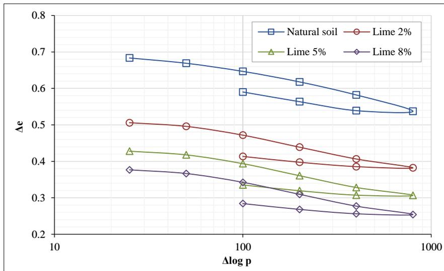
**Figure 11. Variation of void ratio with vertical stress for soil and Lime with percentage (2%, 5% and 8%) prepared at optimum side in odometer test**
