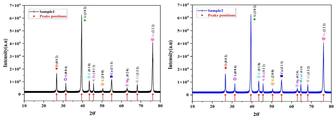
Figure 15. (a) XRD of Natural Soil, (b) XRD of Soil with Lime (CaO) 5%
