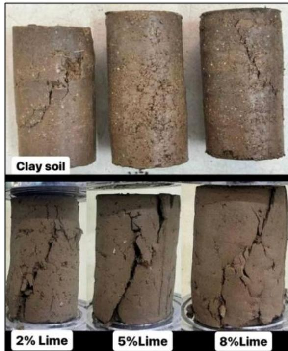
Figure 8. Soil Samples for UCS Test Before and After Lime Addition
