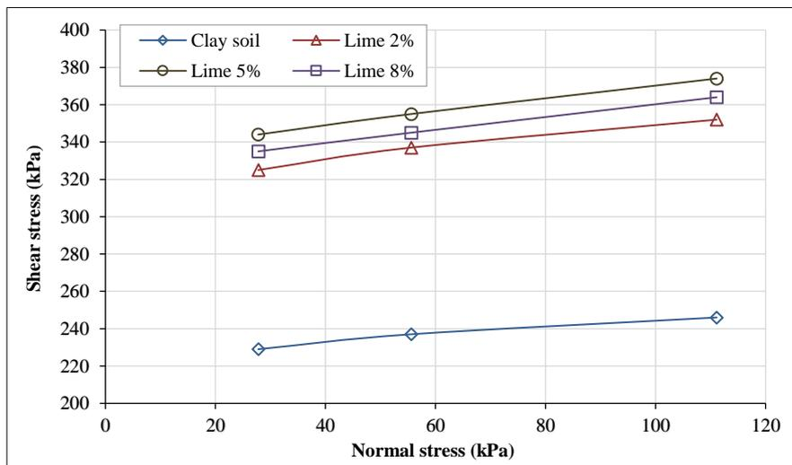
Figure 10. Results of direct shear test of the soil with and without Lime with percentage (2%, 5% and 8%) at optimum sides
