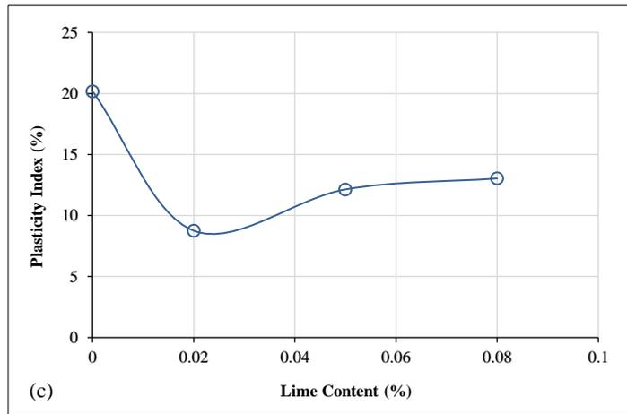
Figure 6. Relationship between (a) Liquid Limit (b) Plastic Limit (c) Plasticity Index and content of Lime
