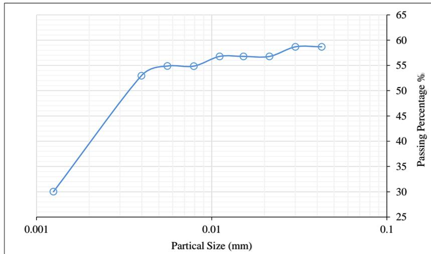
Figure 1. Particle Size Distribution of the Soil Samples Utilized
