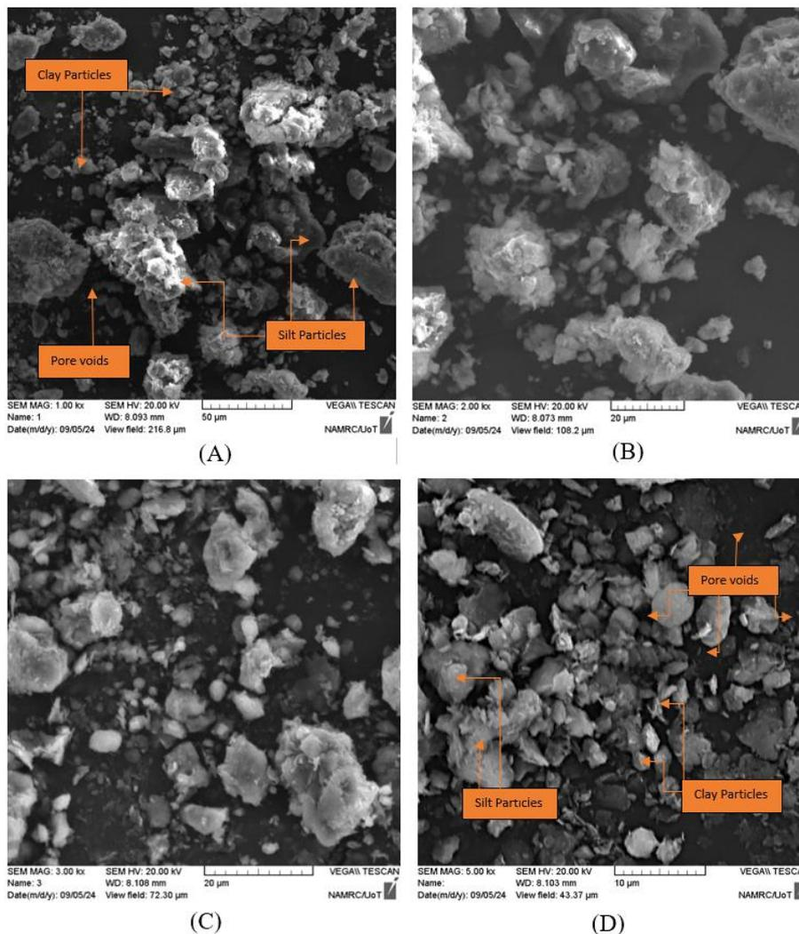
**Figure 13. SEM micrograph of natural soil. (A) Image captured at 1000x magnification. (B) Image captured at 2000x magnification. (C) Image captured at 3000x magnification. (D) Image captured at 5000x magnification**
