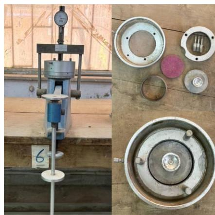
**Figure 12. Oedometer device and cell used**
