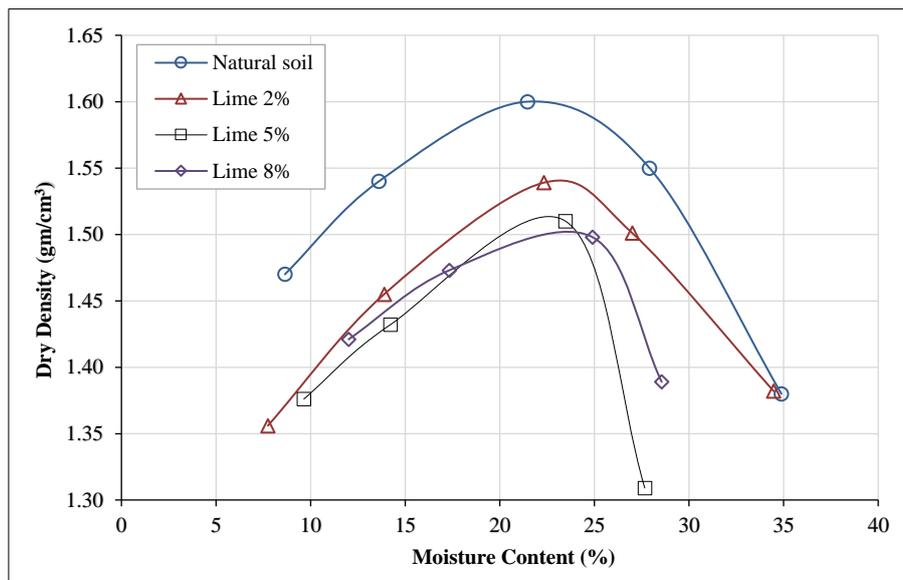
**Figure 5. Compaction curves of natural soil and Lime (2%, 5% and 8%)**
