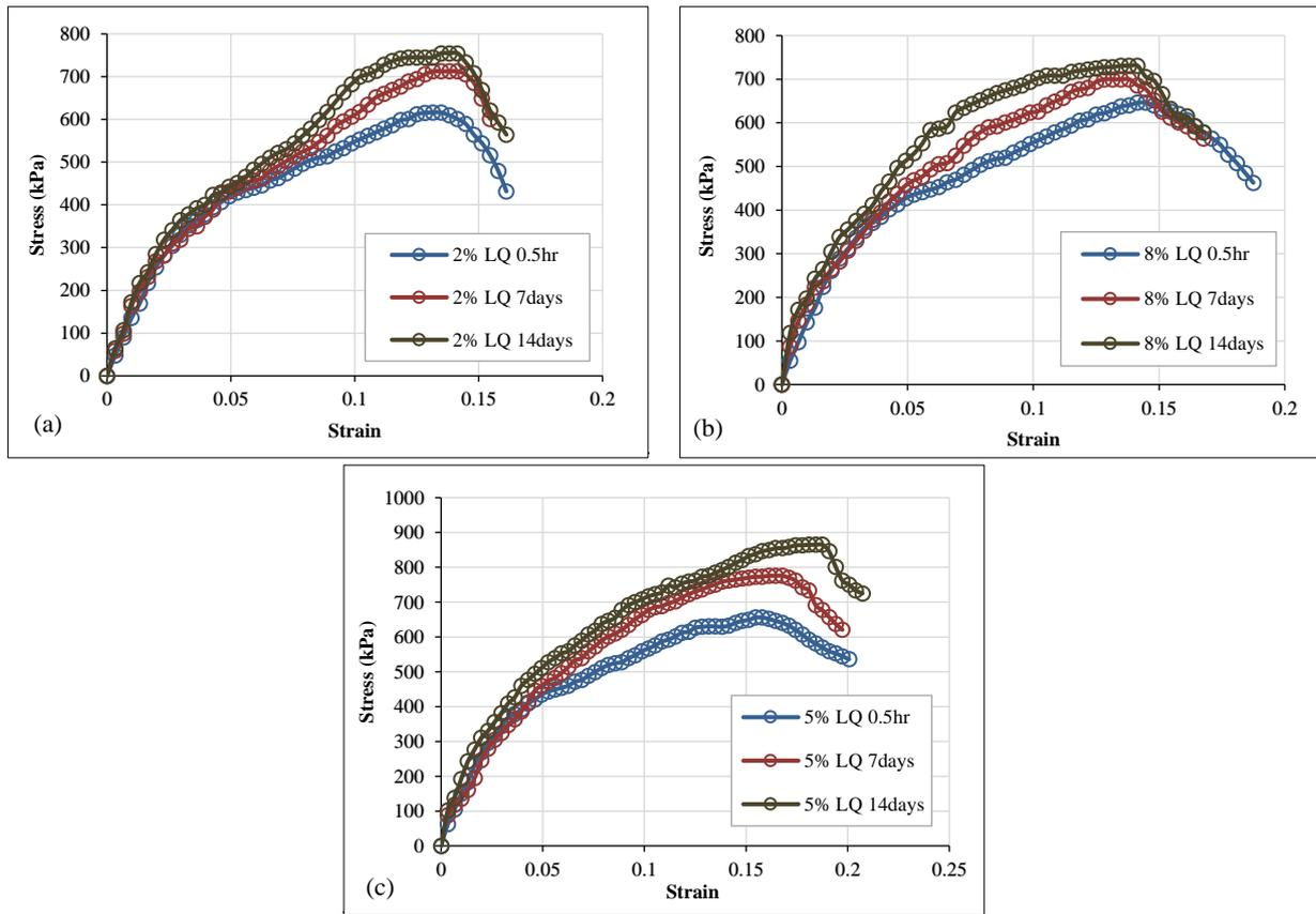
Figure 9. Relationship between the strain-stress curve of natural soil and stabilized soil with (LQ) at different curing time 0.5 hr, 7 days and 14 days (a) 2% LQ (b) 5% LQ (c) 8% LQ
