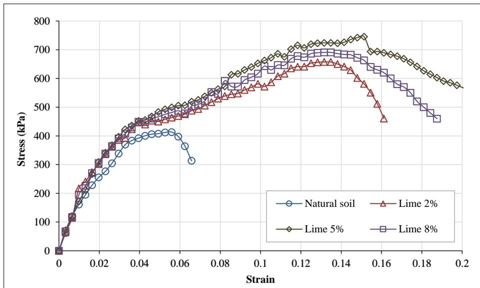
Figure 7. Stress-Strain relationship for natural soil at optimum side with Lime with percentage (2%, 5% and 8%)
