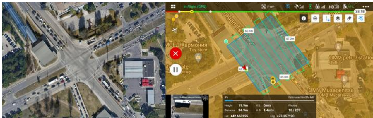
Figure 1. Image of the surveyed intersection and UAV flight plan
