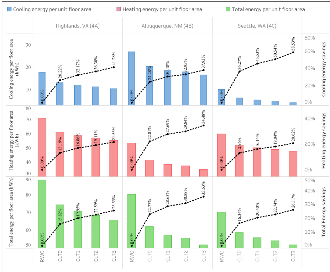
Figure 6. Energy consumption per floor area and energy savings percentage for heating, cooling, and total energy in Climate Zones 4
