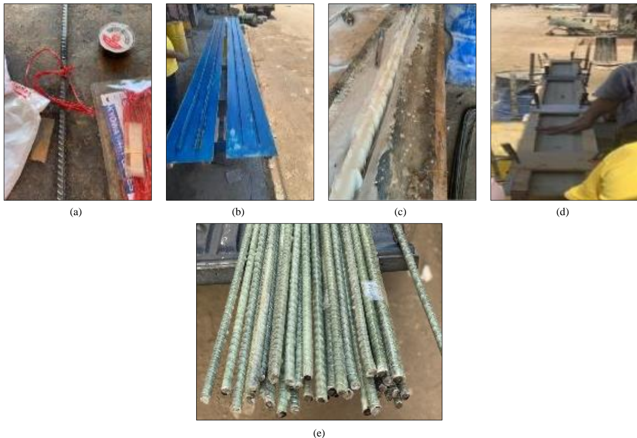
Figure 2. Manufacturing process of the hybrid bars; (a) 10 mm steel core with strain gauge; (b) Wooden form; (c) The steel core with fiber glass; (d) Compacting the wooden form; (e) The bars fully coated with the fiber glass
