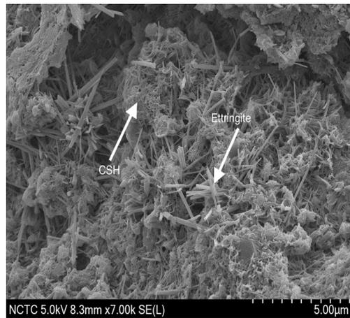
**Figure 11. Scanning electron micrograph of interlocking block BA-20 after 7 days**
