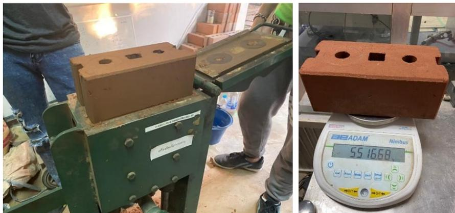
Figure 3. Interlocking block production
