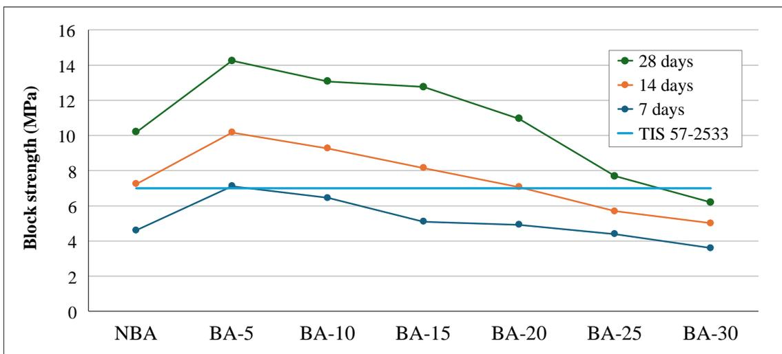
**Figure 9. Compressive strength of blocks with SCBA replacement, where blue horizontal line is TIS 57-2533 strength requirement for load-bearing blocks**
