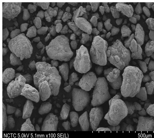
Figure 5. Scanning electron micrograph of lateritic soil
