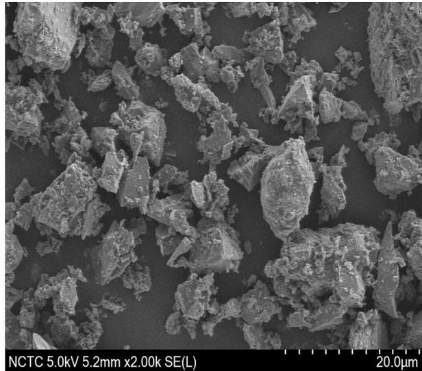
Figure 6. Scanning electron micrograph of cement
