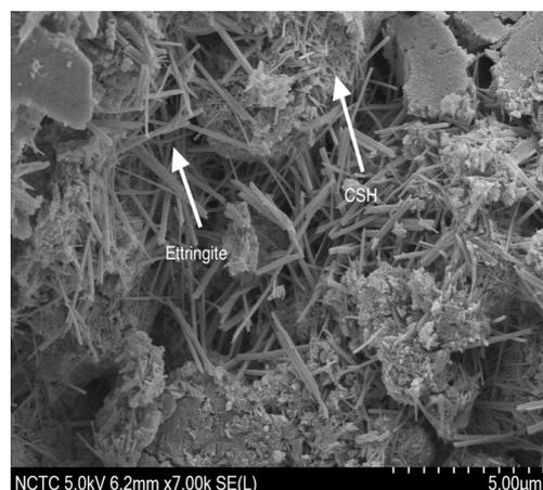
**Figure 10. Scanning electron micrograph of interlocking block NBA after 7 days**
