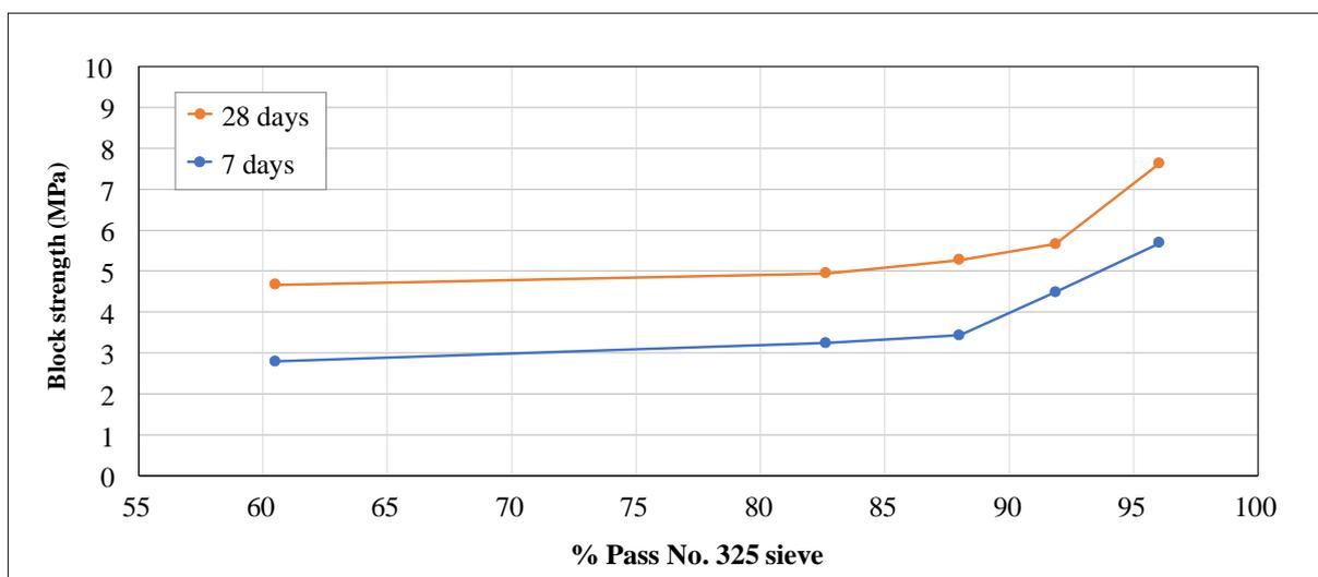
Figure 7. Effect of SCBA fineness (percentage passing through No. 325 sieve) on block strength
