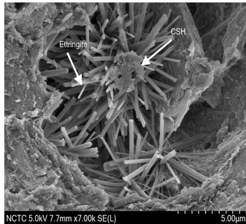
**Figure 14. Scanning electron micrograph of interlocking block NBA after 28 days**
