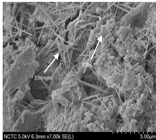
**Figure 15. Scanning electron micrograph of interlocking block BA-20 after 28 days**
