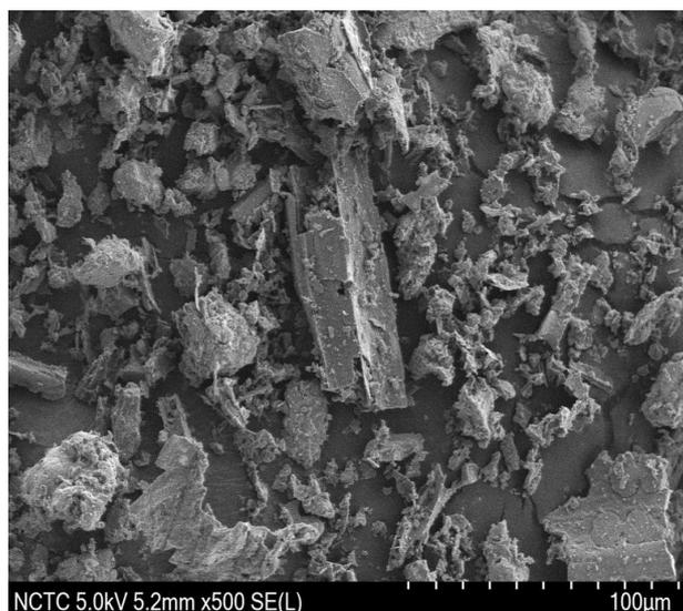
Figure 8. Scanning electron micrograph of SCBA
