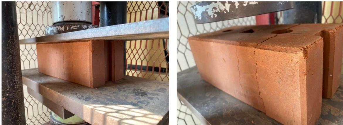
Figure 4. Compressive strength testing of interlocking block
