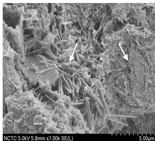
**Figure 13. Scanning electron micrograph of interlocking block BA-20 after 14 days**
