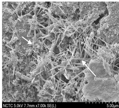
**Figure 12. Scanning electron micrograph of interlocking block NBA after 14 days**
