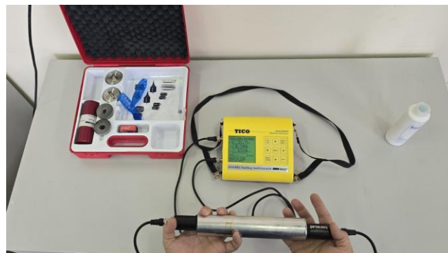
Figure 6. UPV tests on short cylinders
