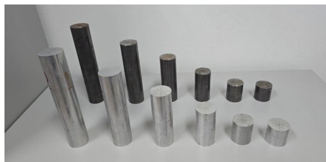
Figure 5. Steel and Aluminium cylinders of six different slenderness
