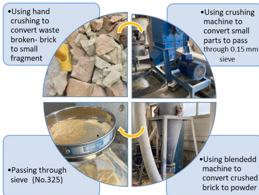
Figure 4. Process of converting waste brick to the powder
