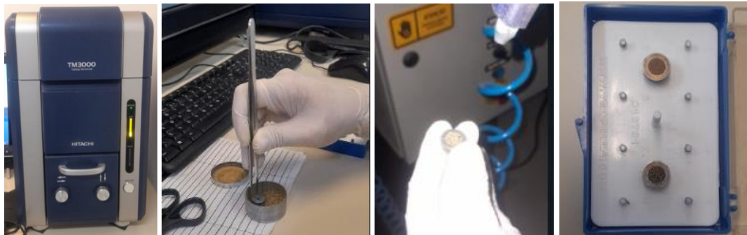
Figure 2. Preparation of Soil Sample for SEM/EDS Analysis
