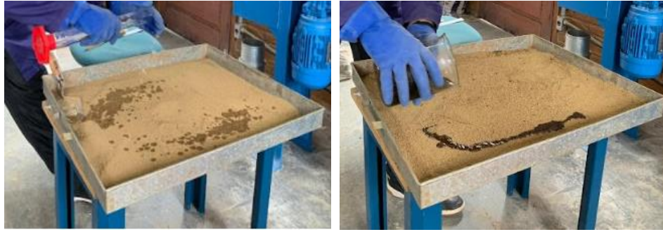
Figure 5. Soil-Emulsion Mixing Procedure
