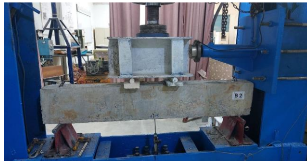
Figure 8. A hydraulic testing machine with a test configuration
