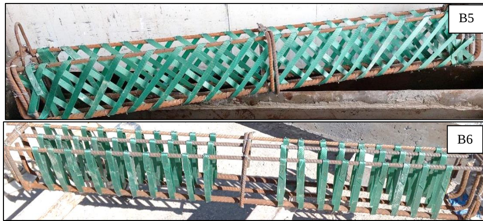
Figure 7. Plastic belts configured as shear zone stirrups (Note: B1R has the same details but without plastic strips)
