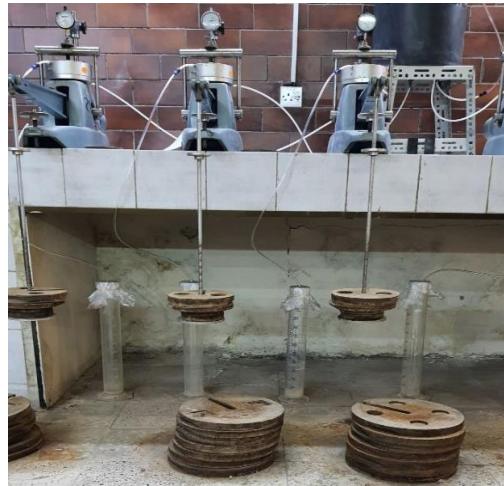
Figure 2. Oedometer permeability leaching test samples
