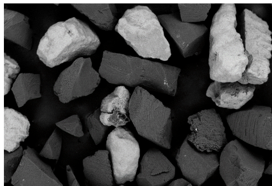
Figure 13. SEM image of the eggshell and sachu inchi cuticle mixture (100X)
