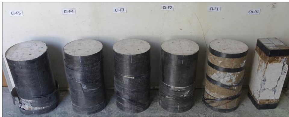
a) CFRP-confined circularized columns Ci-F5–Ci-F1 and control column Co-01
