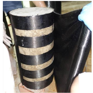
c) CFRP wrapping in progress
