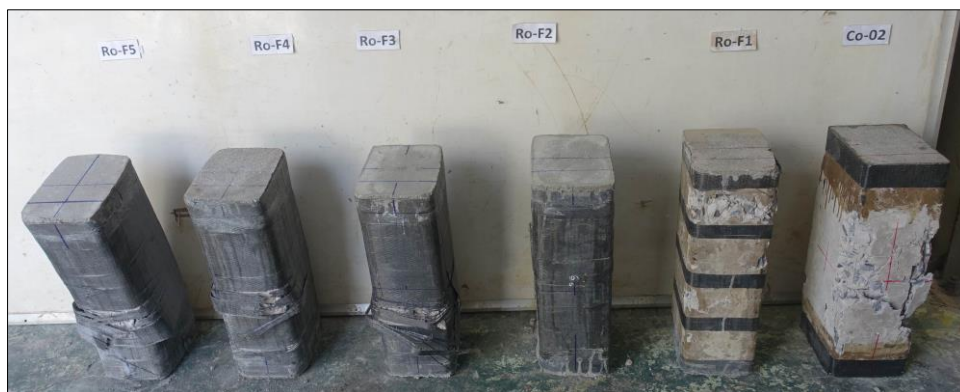
b) CFRP-confined corner-rounded columns Ro-F5–Ro-F1 and control column Co-02
