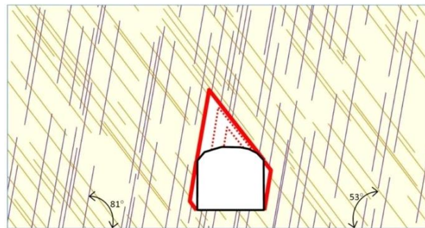
Figure 8. Rock mass fracturing in a trench side of the transportation slope No. 2. fracture systems: 1 m - according to the dip of the rock strata; 2 m - according to the secants; 3 m - cross-sectional
