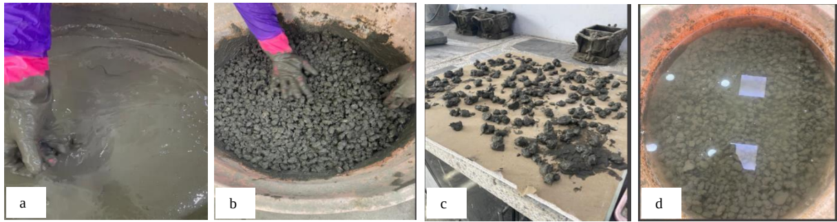
Figure 4. Treatment process: a. Preparing the slurry, b. Treating the RCA, c. Spreading the aggregate, and d. Curing
