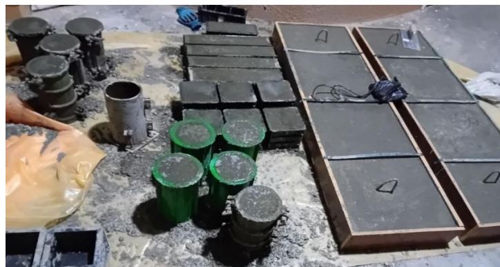
Figure 2. Casting slab and concrete control specimens
