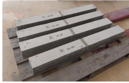
Figure 5. Reinforced concrete beams
