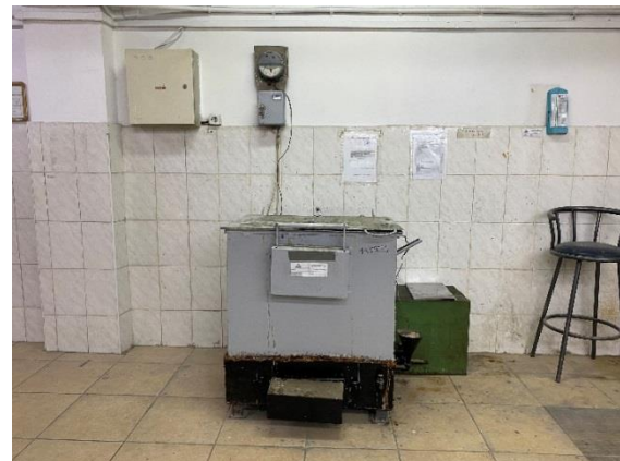
Figure 2. Mixer from the German company "TESTING" with a capacity of 2 liters and a laboratory steam chamber
