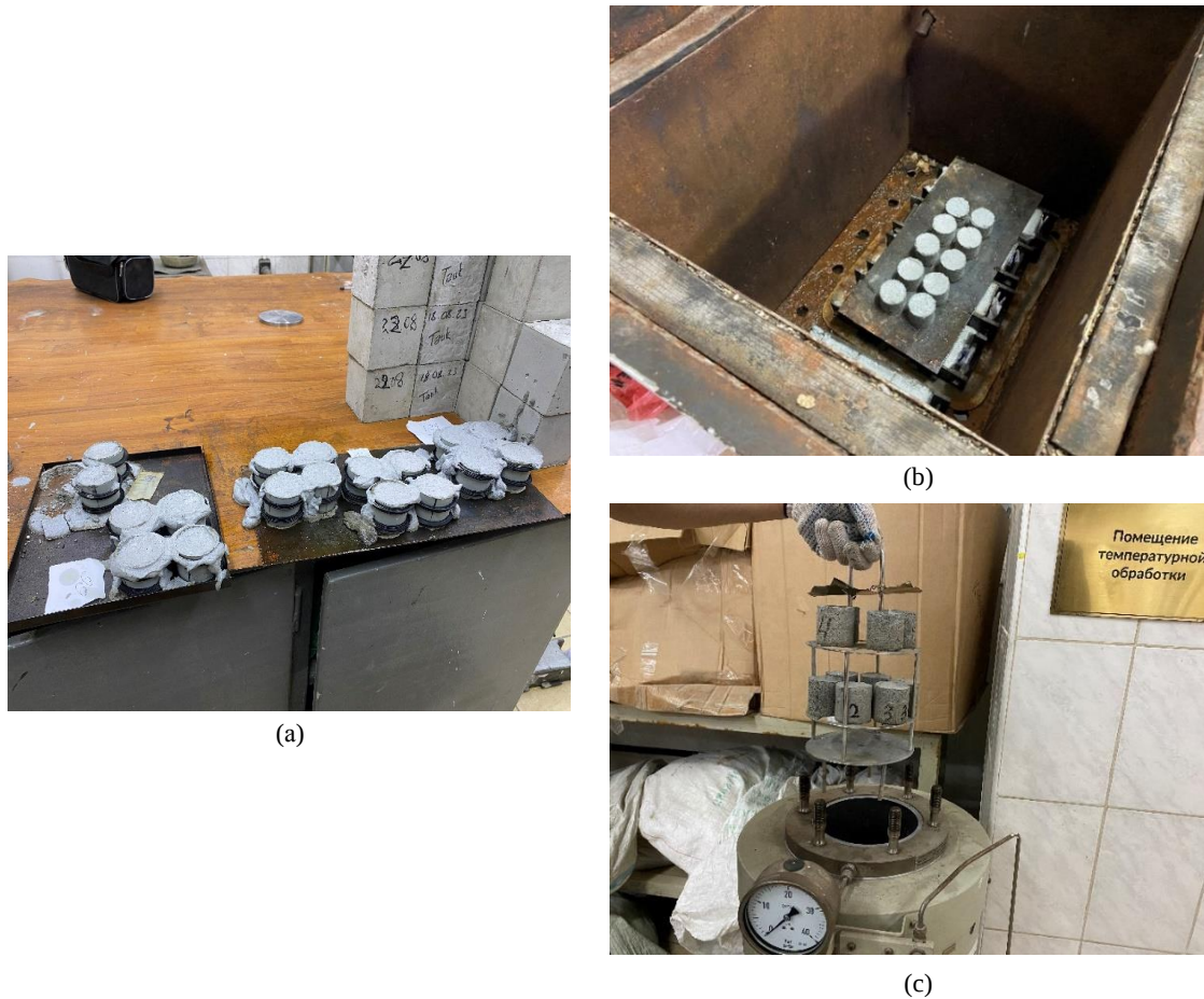
Figure 10. Molded cylindrical samples (a) and placing cube samples and cylindrical samples in a steam chamber (b) and an autoclave (c)
