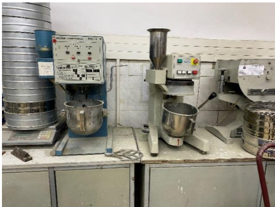
Figure 2. Mixer from the German company "TESTING" with a capacity of 2 liters and a laboratory steam chamber
