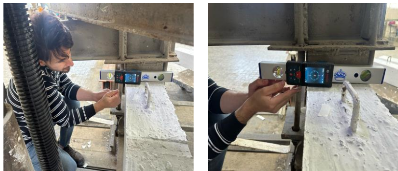
Figure 6. Measurement of Twist Angle
