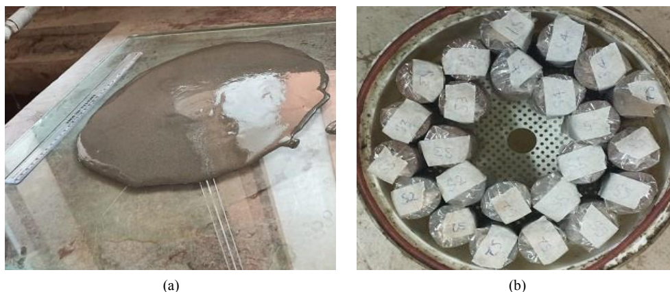
Figure 2. (a) Flowability measurement (b) Sample sealed with cling film and desiccator-cured
