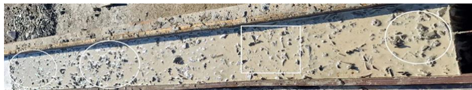
Figure 9. During Casting, Plastic Trash Rises to the Surface
