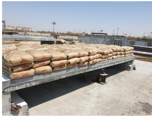
Figure 5. Loading arrangement for structural testing of semi-precast slabs
