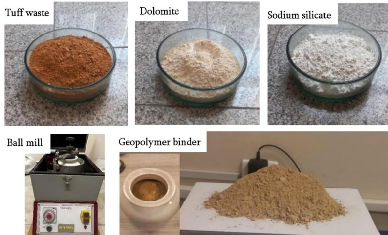
Figure 5. The raw materials for geopolymer binder
