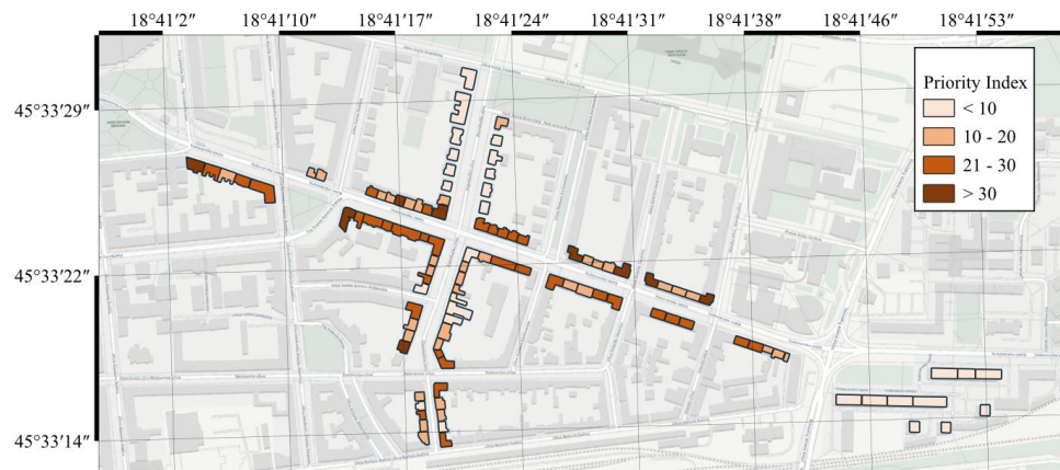
Figure 20. Classification of surveyed buildings according to the Canadian RVS method (for 0.23g ), with priority index levels
