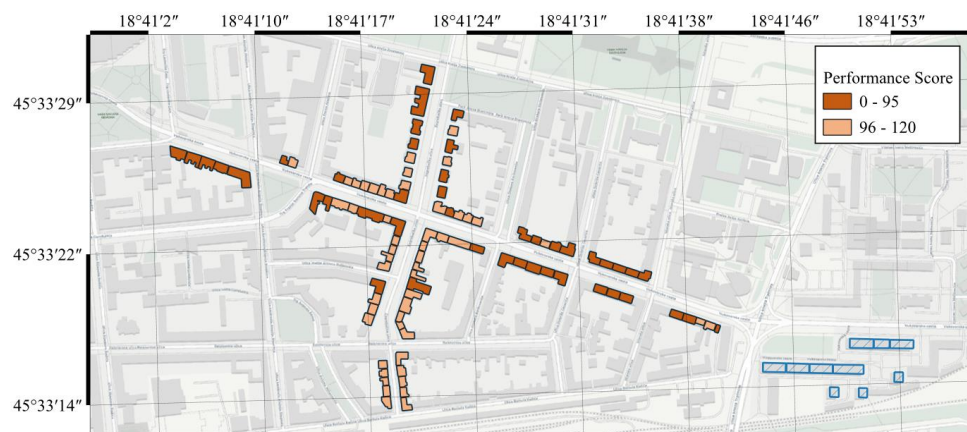
Figure 21. Classification of surveyed buildings according to the Turkish RVS method (for 0.2g-0.4g ), where performance scores are shown with respect to their average value
