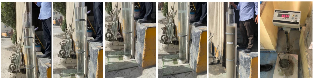
Figure 6. The washout test steps according to the US Corps-C661 [21, 46]
