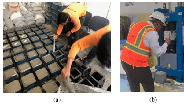
Figure 5. (a) Cubes preparation for compressive strength test, (b) applying the test
