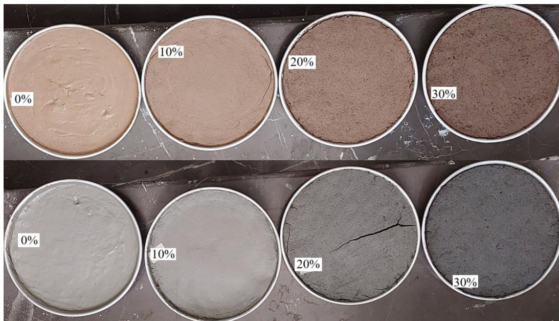
Figure 7. The specimens after 24 hours assembled with minor fracture
