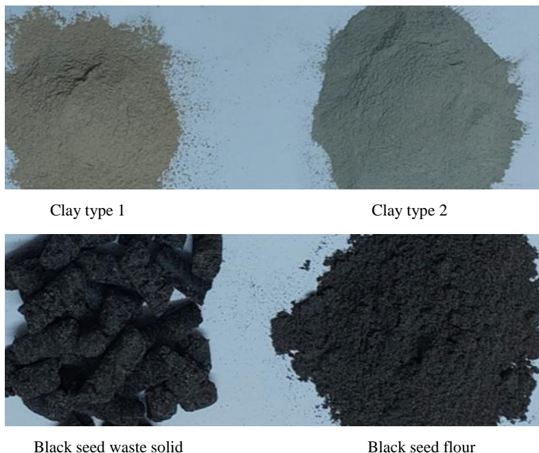
Figure 4. The materials were used for preparing the specimens
