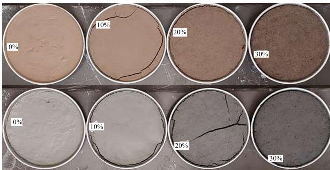
Figure 8. The specimens after 48 hours assembled with fracture
