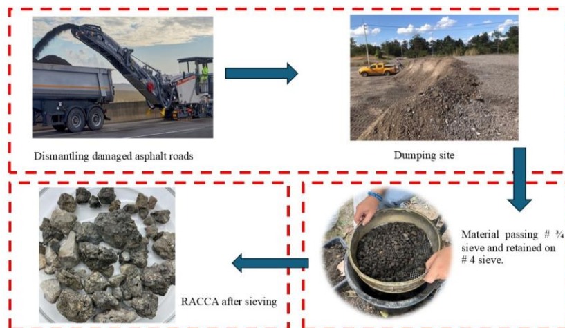
Figure 4. Flow diagram of steps to produce RACCA material passed #3/4 in. sieve and retained on #4 sieve
