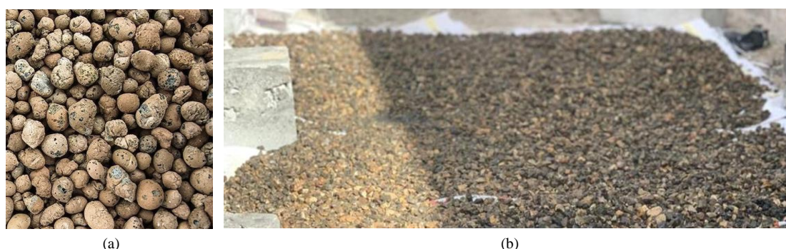
Figure 7. (a) LECA as raw material after at treatment phase, and (b) The drying process of LECA in air
