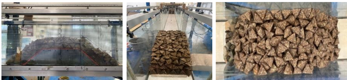
Figure 4. Side, front, and top views of the pyramid-shaped gabion protection layer model in the wave flume
