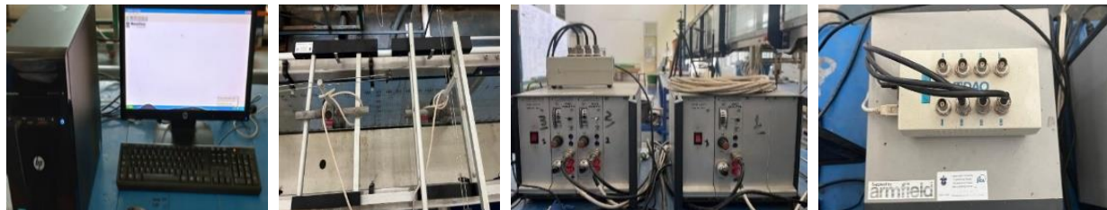
Figure 2. Personal computer unit and oscilloscope software, Wave probe sensor set and buffer, Wave monitor with connecting cable, and Data acquisition
