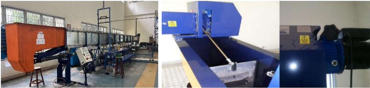
Figure 1. Wave flume and flap-type wave generating unit
