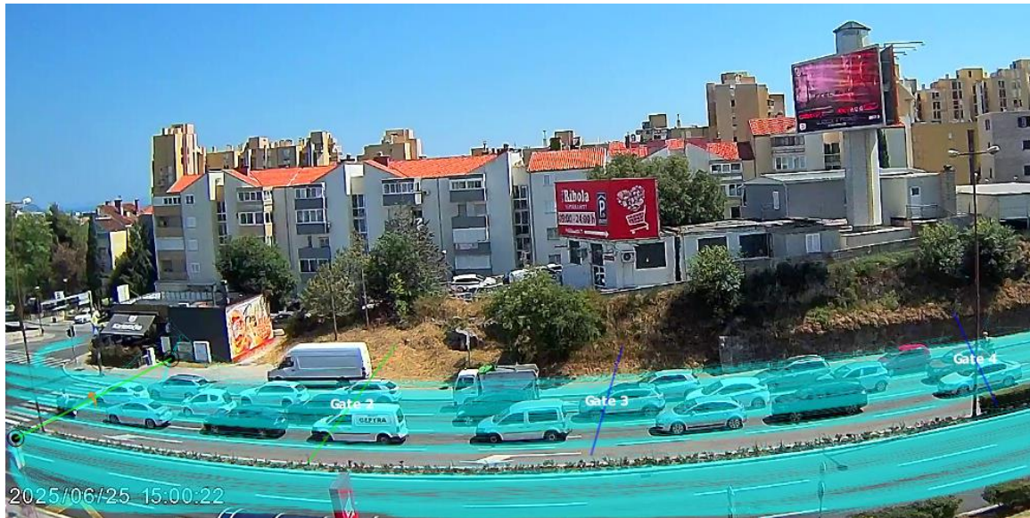
Figure 10. Definition of counting gates and detected vehicle trajectories (DataFromSky)
