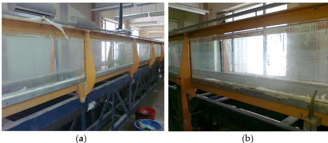
Figure 1. Hydraulic channel experimental workbench: (a) overall view; (b) close-up visualization [19]
